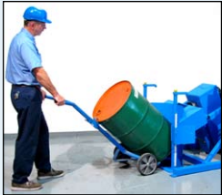
Load upright drum at floor level and secure
